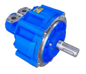
Our SMA heavy duty motor is of radial piston, eccentric configuration. The motor's efficient design includes a hardened high tensile steel crankshaft supported on taper roller bearings. The eccentric element of the crankshaft acts as a hydrodynamic bearing to support the cylinder block and pistons and provides low friction running. The SMA motor range offers displacements from 200 - 16,400 cc/rev.
