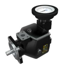
The C range metering pump was designed specifically for the polyurethane foam industry, to provide high accuracy fluid metering with precision flow control and high-pressure capability. The C range pump has capacities from 2 cc to 62 cc per revolution.
