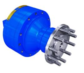
The XF cam motor is of radial piston configuration and is available as a common torque unit or with the option of a shaft or wheel motor housing. The XF motor uses pintle technology to eliminate the need for axial bearing thrust support and to provide a high starting output torque, helping to reduce mechanical losses. The XF motor offers displacements from 150-1,360 cc/rev.
