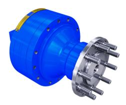
The XF cam motor is of radial piston configuration and is available as a common torque unit or with the option of a shaft or wheel motor housing. The XF motor uses pintle technology to eliminate the need for axial bearing thrust support and to provide a high starting output torque, helping to reduce mechanical losses. The XF motor offers displacements from 150-1,360 cc/rev [9.2-83 in<sup>3</sup>/rev].
