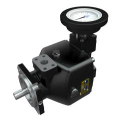
The C range metering pump was designed specifically for the polyurethane foam industry, to provide high accuracy fluid metering with precision flow control and high-pressure capability. The C range pump has capacities from 2 cc to 62 cc per revolution [0.1 - 3.8 in<sup>3</sup>/rev].
