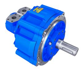
Our SMA heavy duty motor is of radial piston, eccentric configuration. The motor's efficient design includes a hardened high tensile steel crankshaft supported on taper roller bearings. The eccentric element of the crankshaft acts as a hydrodynamic bearing to support the cylinder block and pistons and provides low friction running. The SMA motor range offers displacements from 100 - 16,400 cc/rev [12.2 - 1,000.4 in³/rev].
